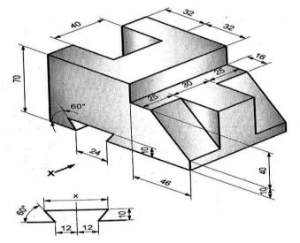
(c) Fig. shows pictorial view of an object. Draw the front view, top view and 5 N side view. Use first angle projection method.
