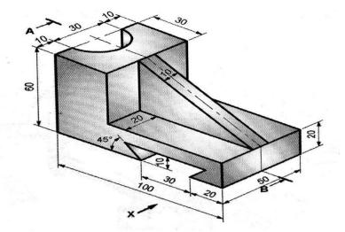
(b) Draw Left side view, elevation, and plan of Figure according to 5 first Angle projection method.
