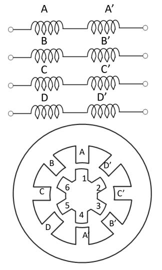
• Four Phase 8/6 pole Variable reluctance type stepper Motor
