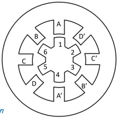
• Four Phase 8/6 pole Variable reluctance type stepper Motor
