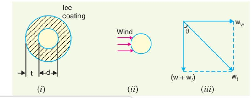
Total weight of conductor per unit length is
