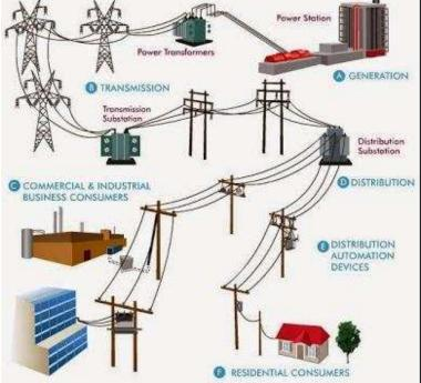
An electric supply system consists of three principal components *viz.*, the power station, the transmission lines and the distribution system. Electric power is produced at the power stations which are located at favourable places, generally quite away from the consumers. It is then transmitted over large distances to load centres with the help of conductors known as transmission lines. Finally, it is distributed to a large number of small and big consumers through a distribution network.
